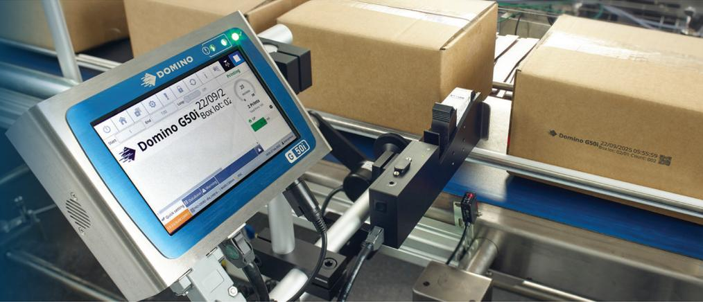
The **G50i** is our entry-level thermal ink jet (TIJ) printer which is an ideal option for those looking for a simple-to-use, simple-to-run system for basic product and box coding.
